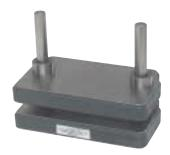
**CAST IRON DIE SETS** are precision surface ground and come equipped with hardend ground bushings, allowing for close tolerance fit. Fine-Grain cast-iron materials are used along with hardened pins for extended wear. (See Page 17)
