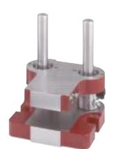
**FLANGED STOCK TWO POST DIE SETS** are stress relieved, blanchard ground, and flame cut. Hardened steel ground bushings are honed to exact tolerance. (See Page 18)
