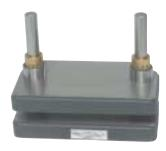
**CAST IRON DIE SET WITH BALL BUSHINGS** are precision surface ground and are made of fine grained cast iron materials. Guide pins are made of case hardened steel, precision ground, and precisely matched for full contact pre-load operation. Ball retainers are gold anodized aluminum. Class chrome alloy balls hold a 25 millionth tolerance and are held captive by four stakes. Bushings are hardened steel ground and honed to exact tolerance. Maximun stroke length is three inches. (See Page 17)
