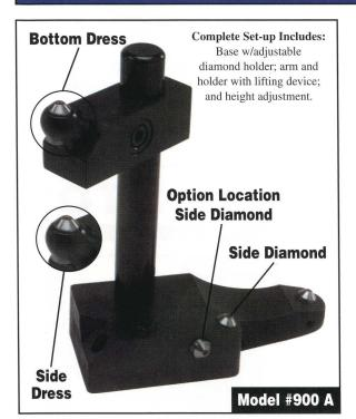
The Handidress is a tool for the toolroom or production department. It is used for the dressing of surface grinding wheels. The tool features a cast iron base and hardened post.
